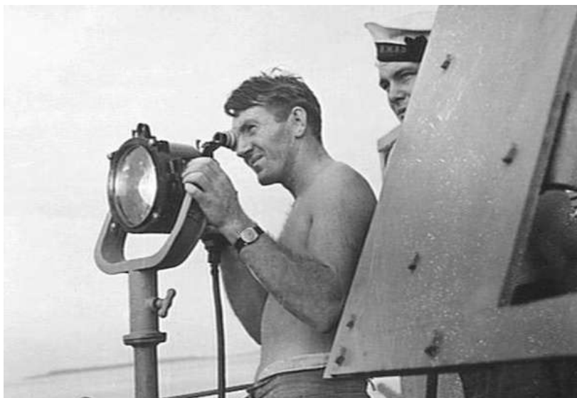
Left: Directional flashing light was routinely used during World War II to pass signals between
