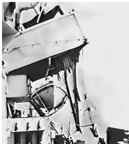
Left: Damaged port wing of the bridge and port motor boat and stanchions
