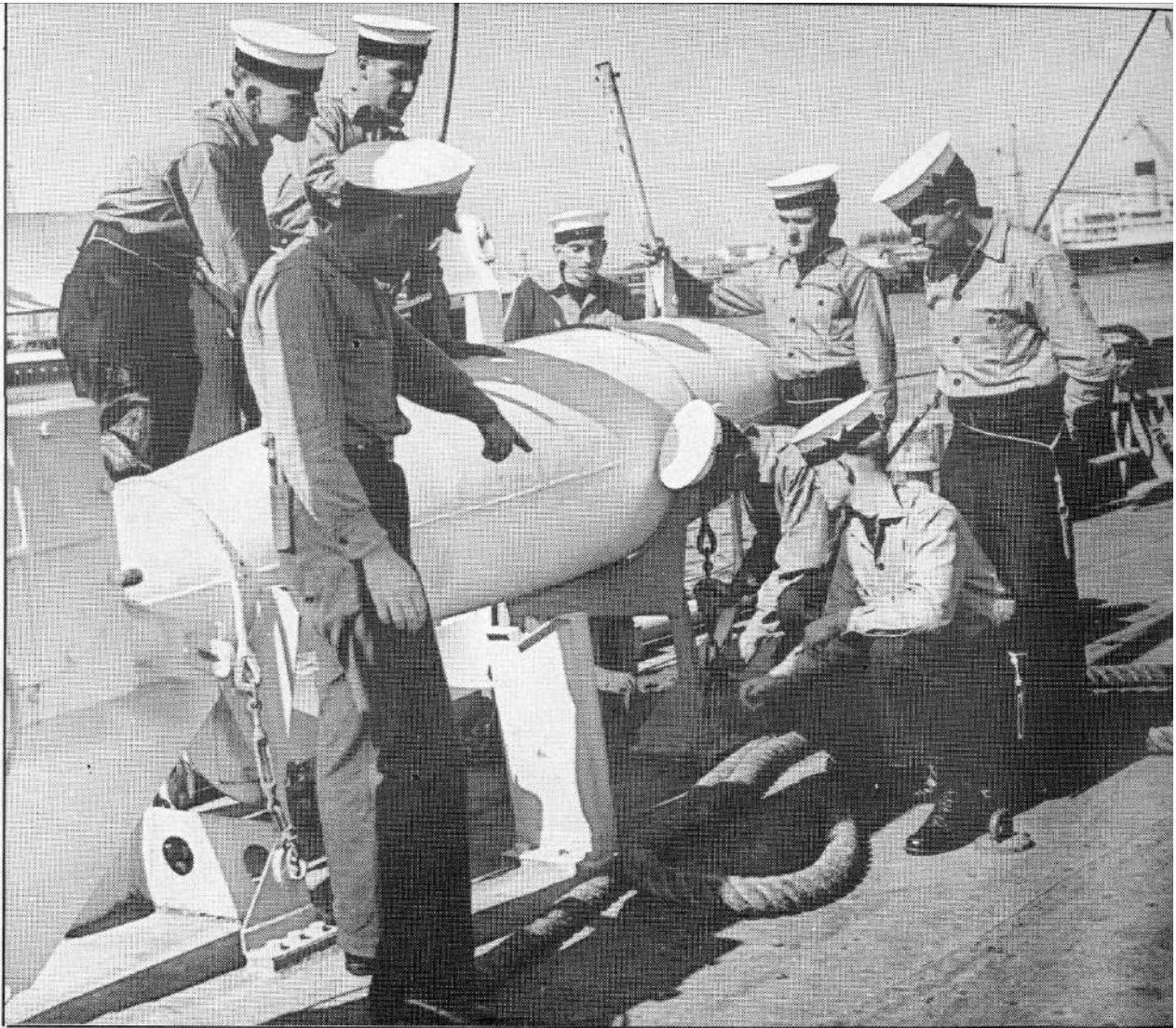
Crew with paravane, August 1951. The Mildura was active after the war sweeping up mines laid earlier to protect Australian waters. Paravanes were towed underwater to sever the moorings of mines. Neg: Navy 45.
