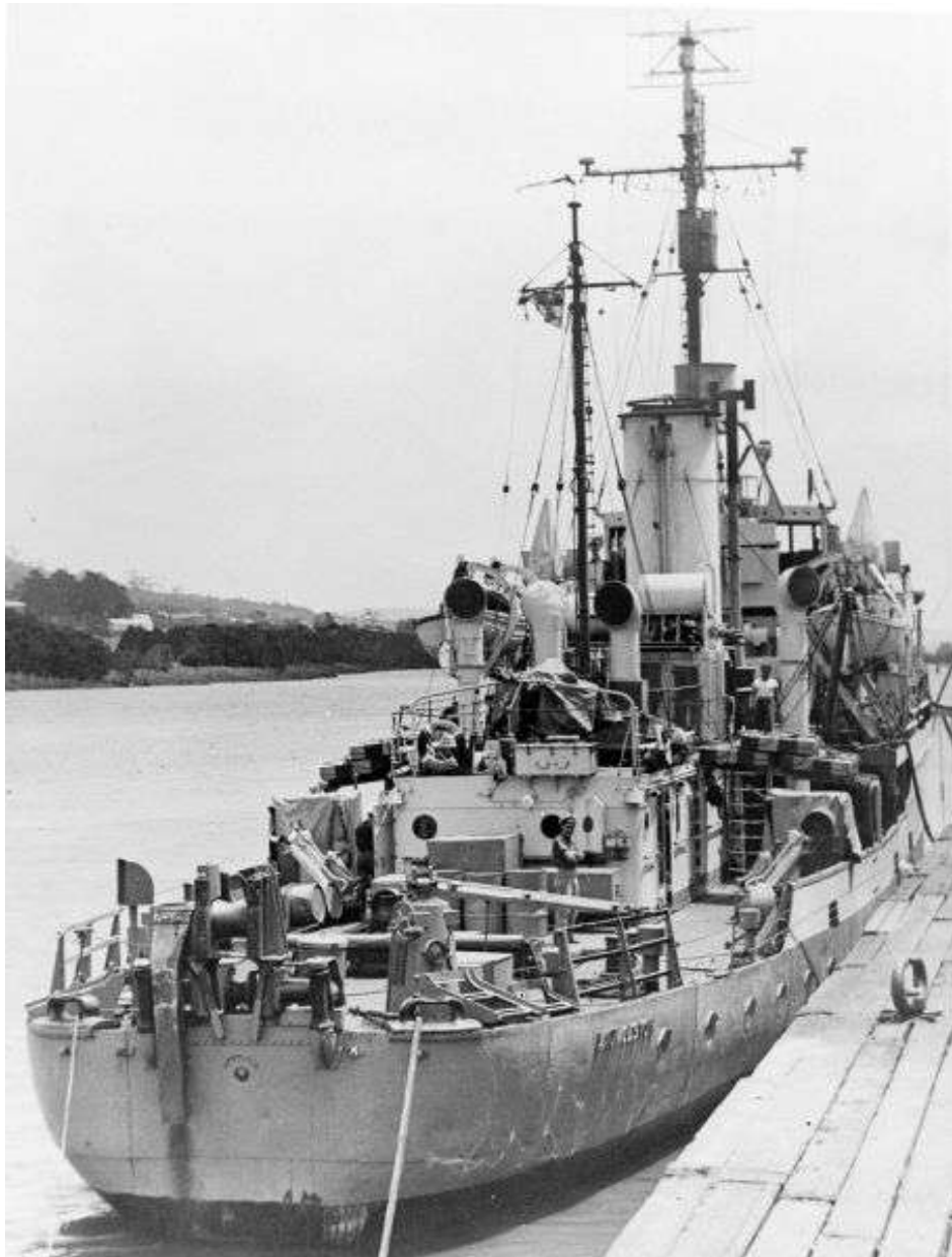
HMAS Launceston as she appeared after being equipped with radar, visible at masthead.
