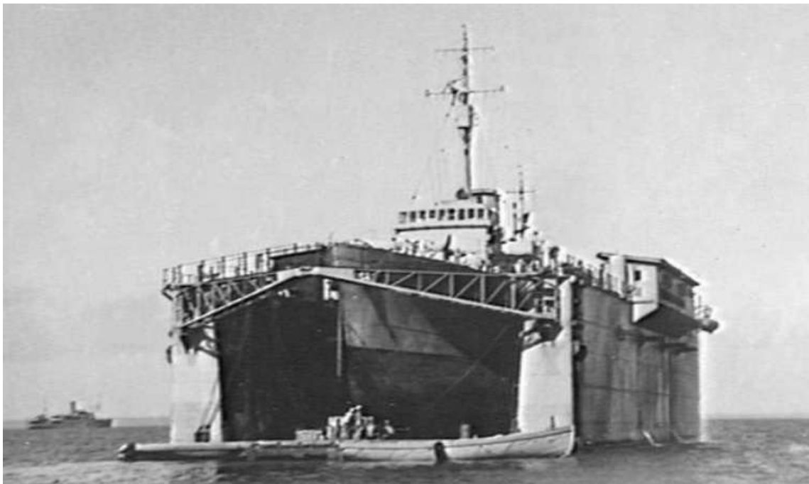
Katoomba secured in floating dock AD1001 in Darwin Harbour following the collision with the US tanker Pecos
