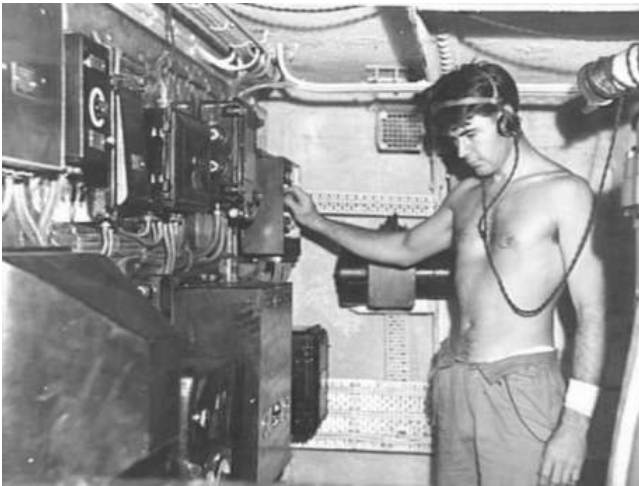
Left: Able Seaman BK Barrow, operating the ASDIC (submarine detection equipment) aboard Geelong (AWM 075741). Right: An engine room artificer operating a small lathe aboard Geelong. (AWM 075744)
