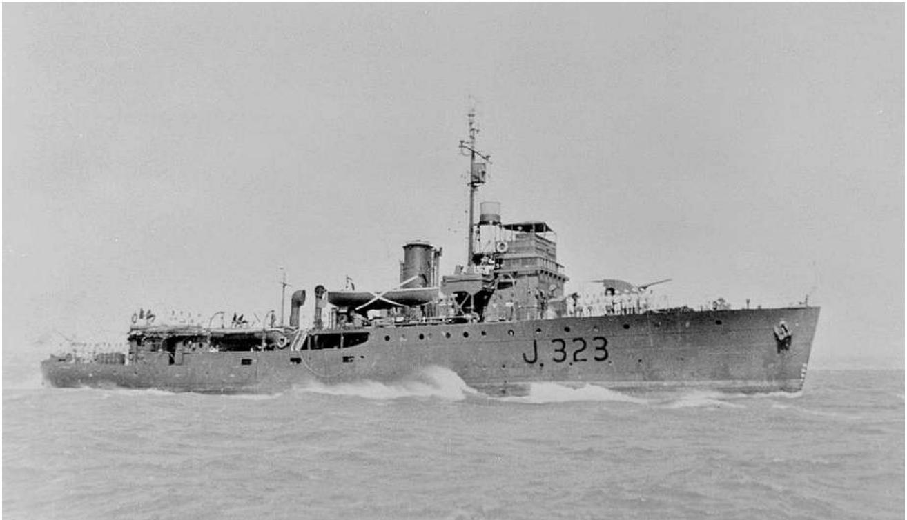
HMAS Benalla differed from her sister corvettes with an additional 'monkey island' fitted above her bridge. In this photo, taken later during the war, types 271 and 291 radar can be seen mounted at the base of the foremast and at the masthead.
