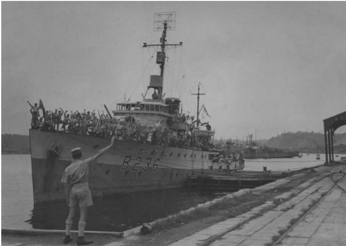
HMAS Ballarat wearing her British Pacific Fleet pennant number, Yokosuka Naval Base, circa 1945. Note also the type 271 radar at the foot of the foremast and the type 291 radar aerial mounted at the masthead.
