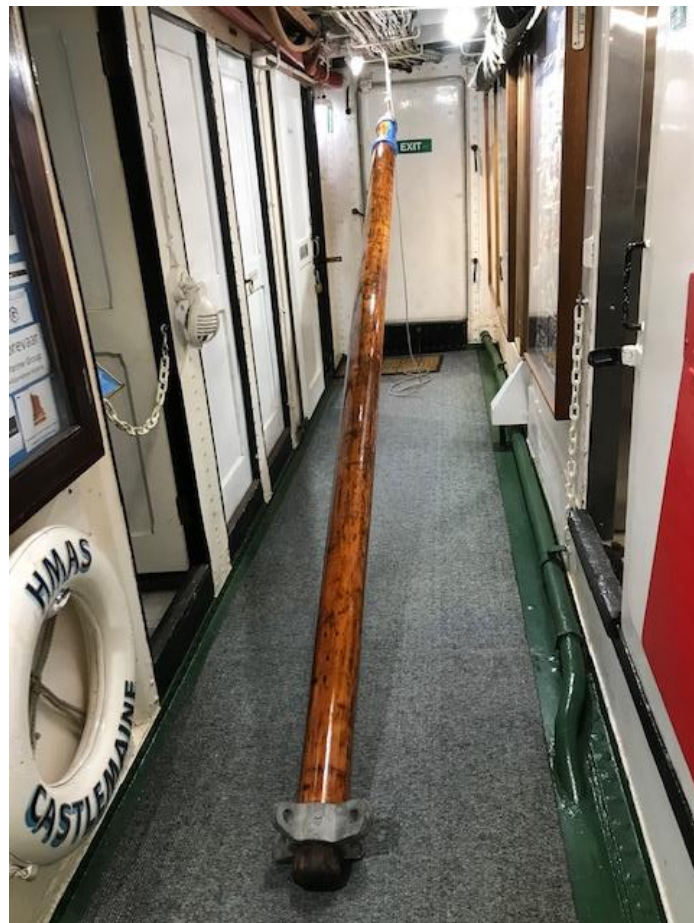
The derrick is made from Hoop Pine and still needs another three coats of lacquer.
